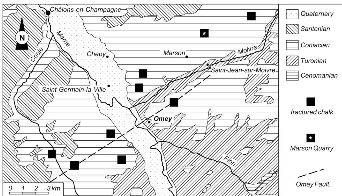
Fig. 2. Geological map of the Omey area with location of the Marson Quarry (modified after Coulon and Frizon de Lamotte, 1988b). The chalk is fractured in a 6-km wide N060°E zone which follows the trace of the Omey Fault (northern border of the Mayence-Sancerre Fault Zone).
